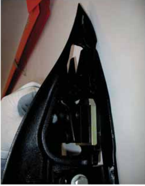
5. Position outer shoe as shown below the bar back 6. Position the knife guide plate on top of bar back as shown
