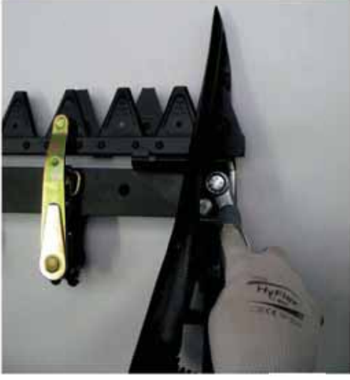
7. Slightly tighten bolts that hold on the outer shoe and set the required clearance of approx. 0.04 - 0.08 inch between the knife guide plate and knife back. 8. To finish, completely tighten bolts
